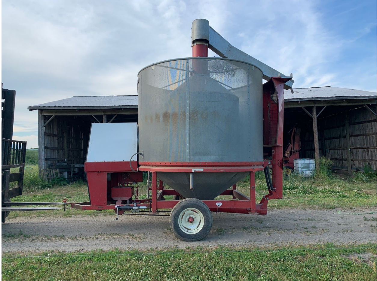
Mobile GT245 XL Mobile Batch Dryer at Lakeshore Farm
