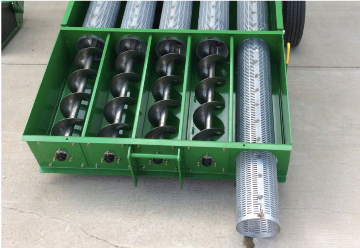
Removable bearing plate on the Kwik Kleen for quick screen changes
