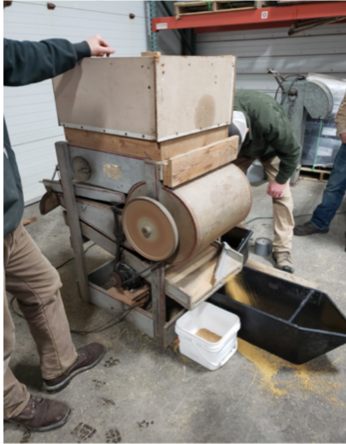
Figure 3: Seed-A-Way screen cleaner for separating wheat
